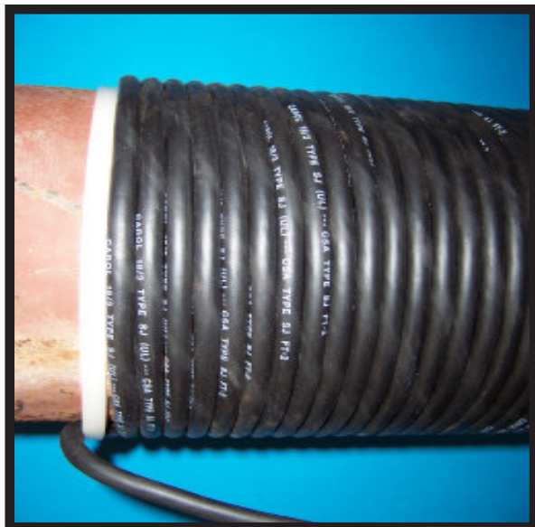
Photo 4a & 4b - Examples of tightly wrapped coils
