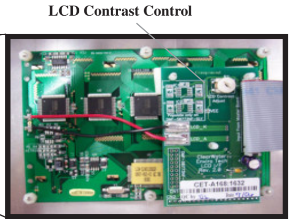
Close-up of LCD Display Board showing the Contrast Control
